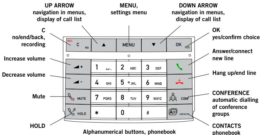
① Some OmniTouch 4135 IP have a different keypad with other symbols. This does not affect the functions of the buttons.
